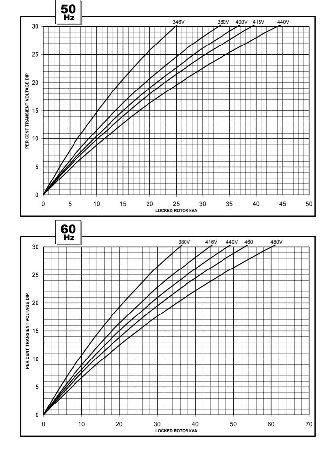
Locked Rotor Motor Starting Curve
